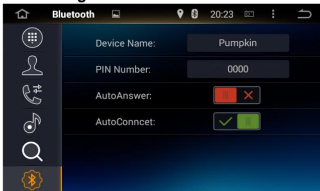
In this menu, you can modify the Device Name, pair pin number. Automatic pairing with phone is defaulted. When the system displays the successful pairing is done, the phone starts to connect with the connection password of “0000”, and the Bluetooth function is available when the system prompts the successful connection (Bluetooth symbol in the upper right corner of the screen changes from gray to white).
