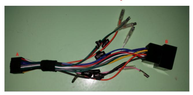
Following the photo above, the A side will be connected to <a href="Pumpkin head unit">Pumpkin head unit</a>, the B side will be connected to your car's plug which used to connect to your original car radio.
