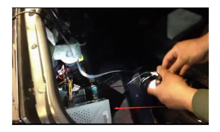
The NO.1 plug is used for Canbus signal output from your car to our unit.
