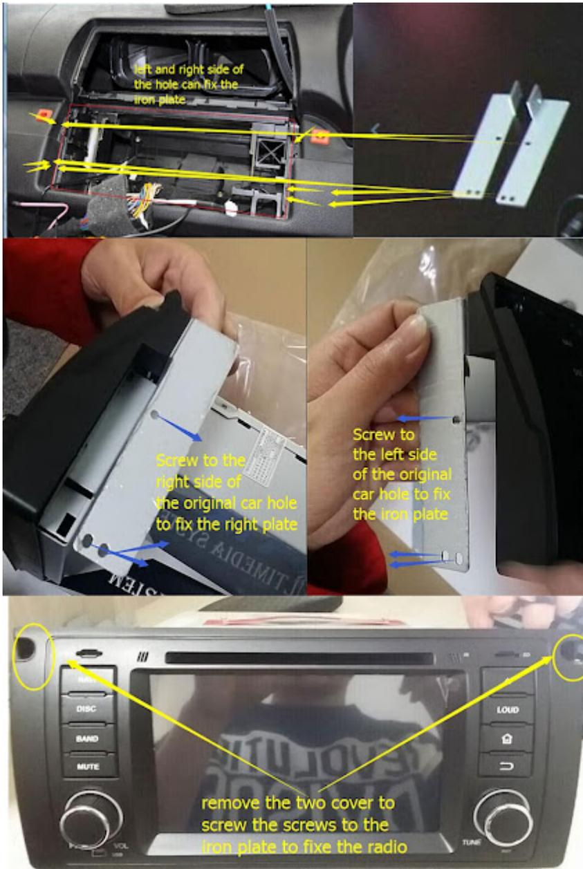
If your BMW X5 E53 comes with factory navigation system, there's a large screen in the dash, the 17pins(before year 2002) or 40pins(after year 2002) plug is not at the back of your factory radio, it's located under the trunk, so you need to use a 5m long power cable with 17pins or 40pins plug to connect the correct plug under the trunk.
