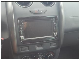
Almost all of <u>Pumpkin universal Andorid</u> car GPS DVD supports the Steering Wheel Control if your car came with this control from factory, but it only supports resistance ladder type since <u>Pumpkin</u> universal head units only offer standard ISO power cable which has no Can-Bus decoder. And the program is easy.
