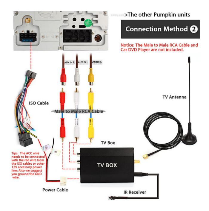
And now we also have some newly listed item which with the rear side like the following link shows, you can use the convert cable which is standard include into the digital tv box to connect. You can also operate and control the TV box on the headunit screen, and the TV box gets power from the headunit.
