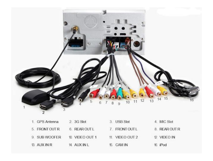
you may connect the digital TV box like this, but you can not operate and control the TV box via the touchscreen of the headunit, you can only use the remote control of the TV box to do that, and the headunit only works as display monitor. And you may need to connect the power lead of the TV box to give power supply to the TV box.
