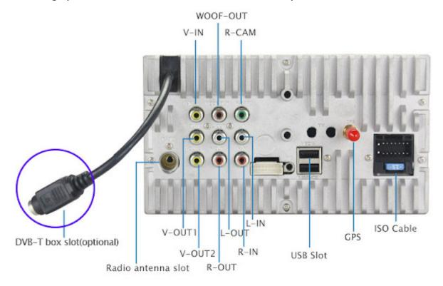
you may connect the digital TV box like this, and you can also operate and control the TV box via the touchscreen of the headunit. And the TV box gets power from the headunit, so you do not need to wire extra wire to get power for the box.
