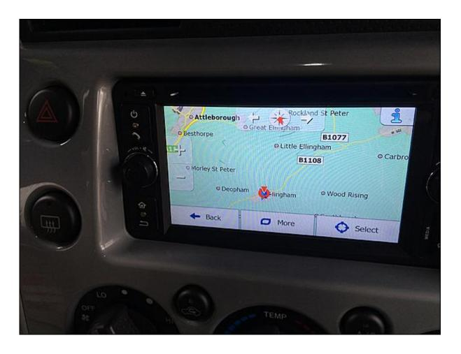
1. Check if other settings such as radio, date and time can be saved or not. If all these settings can't be saved, then you might have plugged the Red ACC cable and Yellow memory wire (labeled with B+ ) into the wrong position. Thus, there is no memory and the Android 4.4 car stereo has no data to save. All you need to do is plugging them in the right position and the setting issue will be
