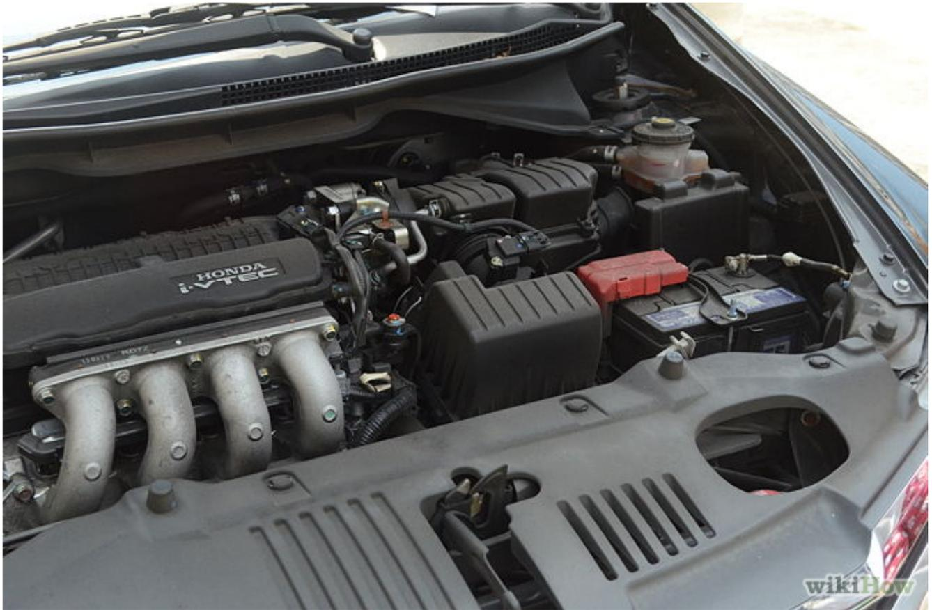
2. Disconnect the vehicle's battery by pulling off the negative cable. Wire the camera to the battery according to the instructions provided with your kit. The battery acts as the camera's power source
