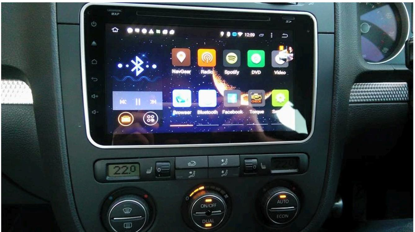
3. Install your rear-view camera monitor. There are several possible locations to install the monitor. The most common locations are on the dashboard or sun visor. The monitor will allow you to view anything behind your car before you back out, so it should be placed in a location that is convenient when driving.
