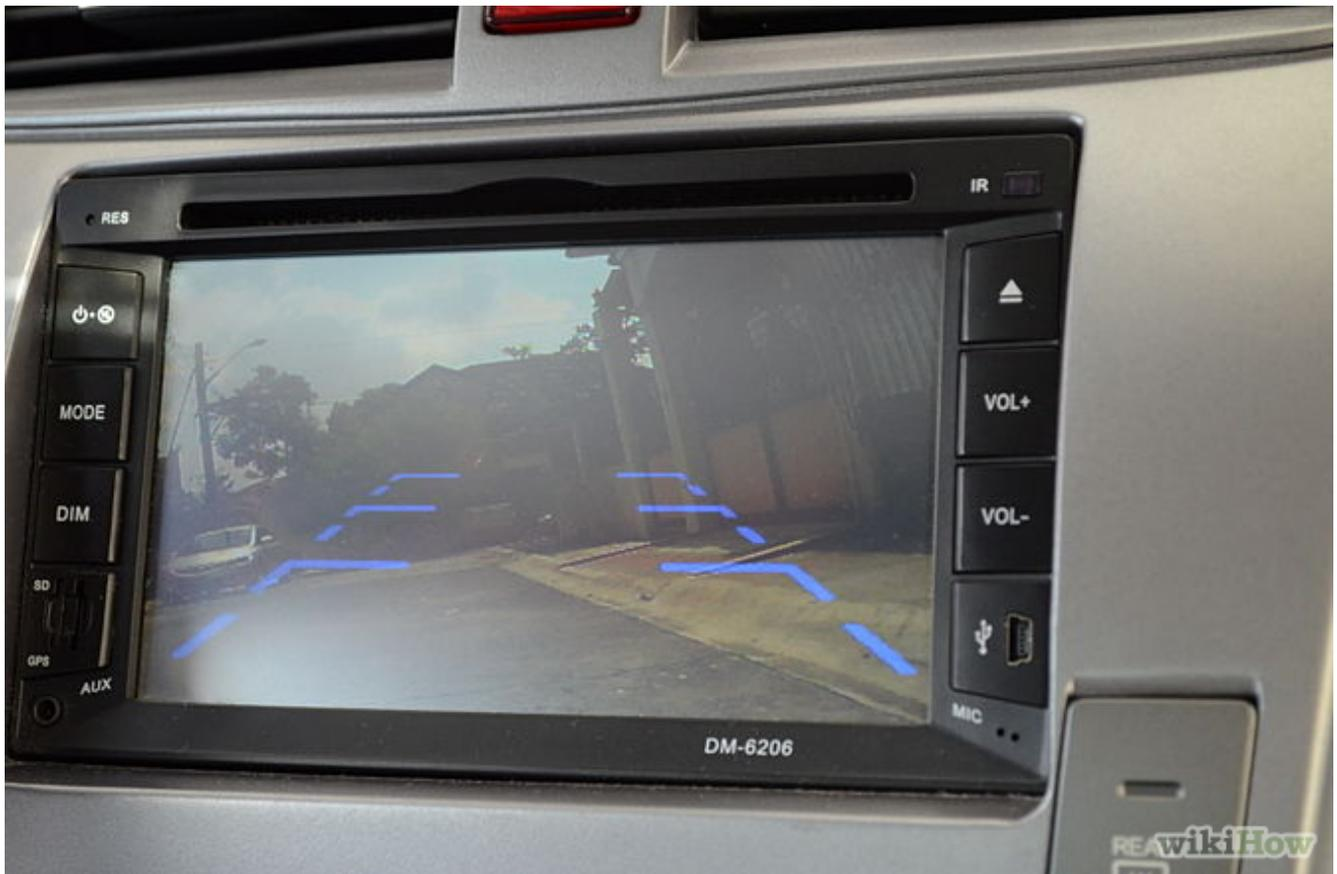
5. Test the camera before attempting to drive with it. Make sure you can clearly see what is behind the car. Turn on the camera and monitor, place an immovable object behind the car, put the car in reverse but keep your foot on the brake, and verify that you can see the object in the monitor.
