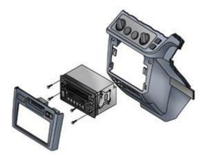
Four bolts and a pair of side brackets attach the stereo to th
