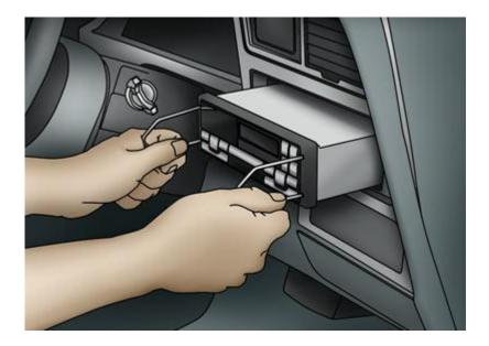
These DIN tools are used to remove the factory stereo from a 2 000 Ford Expedition.
