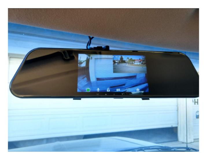
While in the Playback mode, all the various folders are accessible for front and rear recordings. These include loop recording, locked files due to impact, files due to motion close to the vehicle when parked. Only front view photos can be accessed in the Playback mode. If you take the TF card to a computer, there is also a photo from the rear camera.
