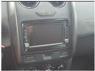
Almost all of <u>Pumpkin universal Andorid</u> car GPS DVD supports the Steering Wheel Control if your car came with this control from factory, but it only supports resistance ladder type since <u>Pumpkin universal head units only offer standard ISO power cable which has no Can-Bus decoder. And the program is easy.</u>
