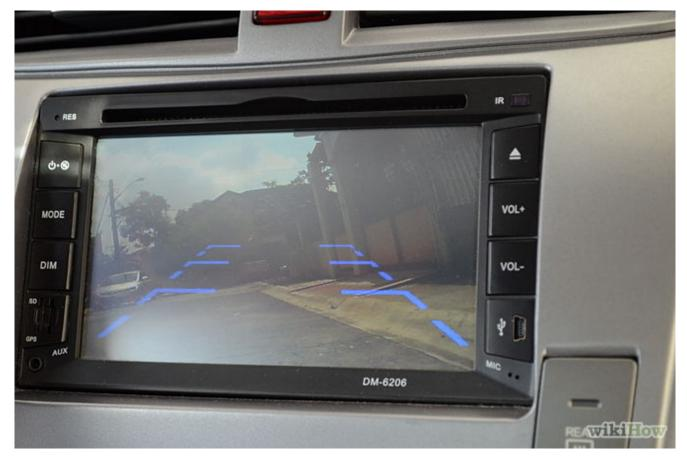
5. Test the camera before attempting to drive with it. Make sur e you can clearly see what is behind the car. Turn on the came ra and monitor, place an immovable object behind the car, put the car in reverse but keep your foot on the brake, and verify that you can see the object in the monitor.
