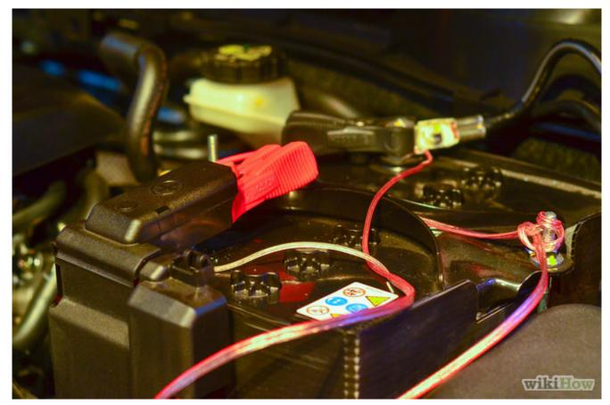
2Disconnect the cables from the vehicle's battery. Raise the hood and locate the vehicle's battery. Verify the correct sized wrench or socket and remove the terminal attaching the battery cables to the battery. Disconnecting the battery will help ensure your safety, and protect the electronic components of your vehicle from short circuits.
