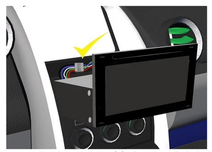
6:Connect the other end of the wiring harness to the back of the car DVD player. Connect the antenna cable to the antenna input on the back of the car DVD player.
