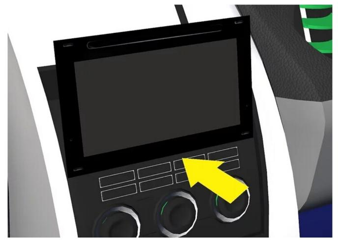
7:Insert the car DVD player and the installation kit in the car's dash. Put in any screws that are required and replace any dash panels that you removed.
