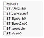
Copy those extracted files into an empty (micro)SD card, and insert to GPS/Navi slot of HU, turn on the car power of the radio, while entering the radio, it will read the update card and automatically update. If the radio is already on, you can use a sharp pen to press RST hole on the radio to reboot and update, the result is the same.
