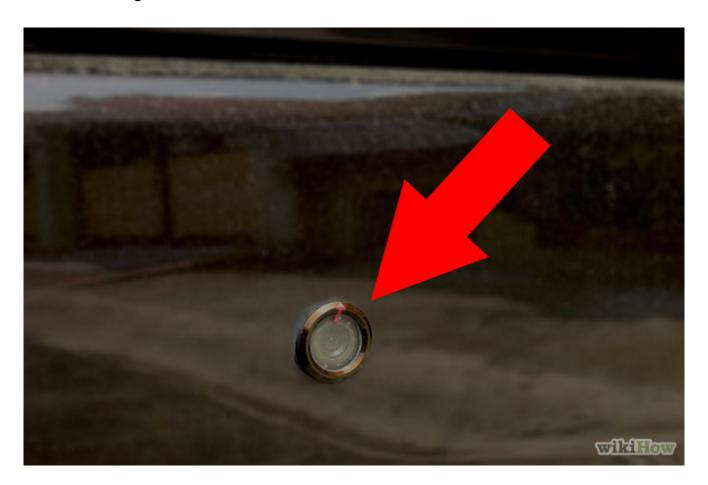
4. Use a drill to install the camera. Mount the camera on the bumper, license plate, or other location at the rear of the vehicle. The kit will include all the necessary mounting hardware. Attach the camera's power wire to the back-up light power wire on your car. If you purchased a wireless camera, you do not need to wire the camera. Reconnect the car battery.
