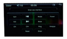
Push a button on the steering wheel controls, followed by the corresponding button on the head unit. Repeat this process until all required buttons are programmed.
