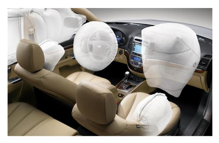
Even the least expensive cars these days have at least two front airbags. In the event of high-speed or high-impact collisions, airbags are only second to seat belts in saving the lives of front seat passengers. The latest auto
