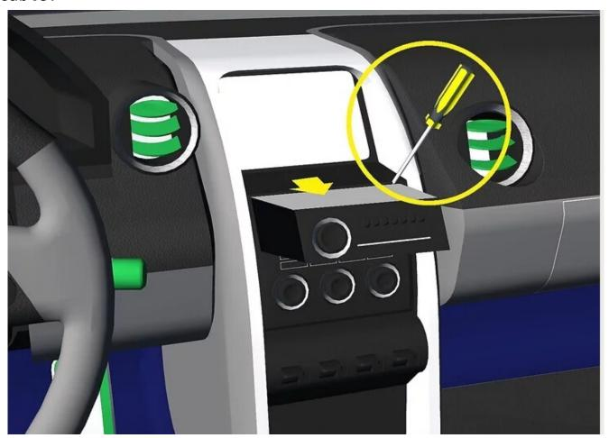
2: Using the proper screwdriver, take out the screws holding the factory stereo in your car's dashboard, then remove the stereo from the dash. You may have to remove parts of the dash to take the stereo out.
