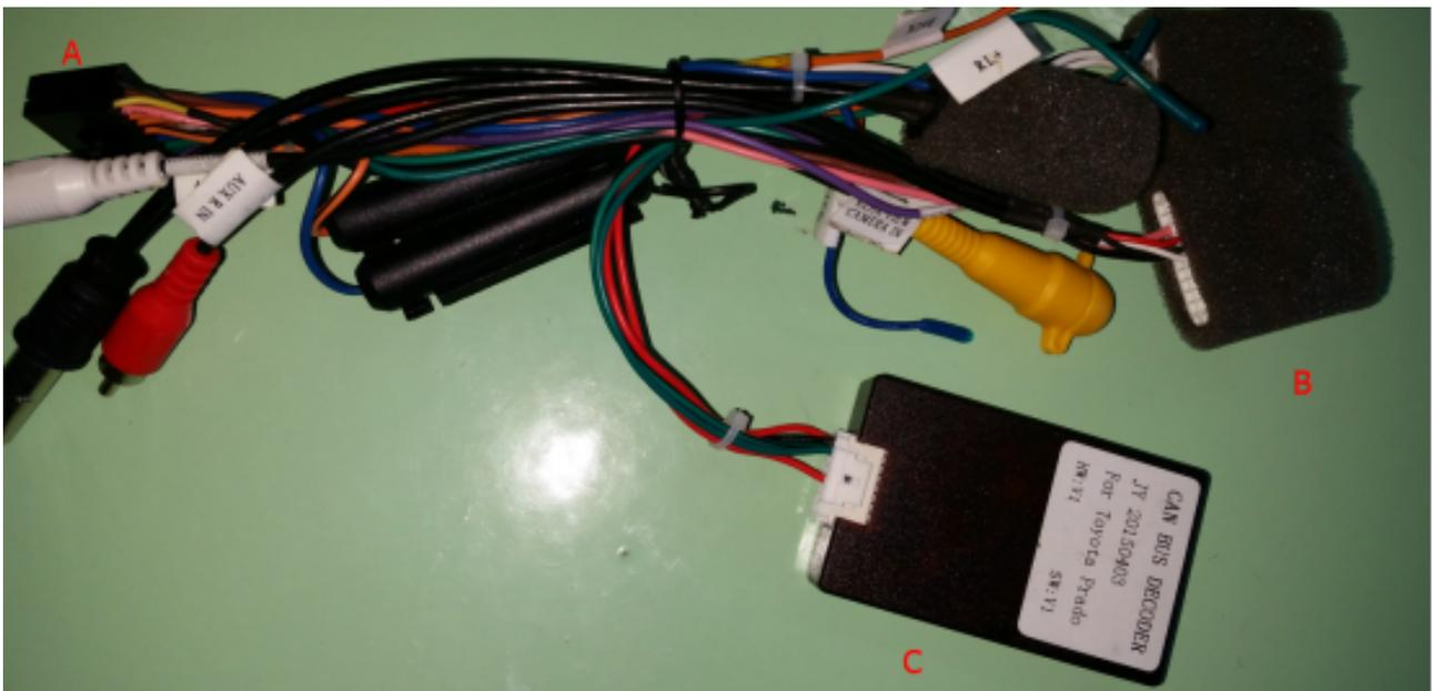
A side connects to Pumpkin autoradio dvd gps, B side connects to your car's plug, C part is the CANBUS decoder we're talking about. This CANBUS decoder controls the SWC, Turning-on/off of the head unit, parking sensor, car on-board computer and so on. Let's say it will decode and transport signal to reverse cable when the car's reversing, then the head unit can show the reversing image.
