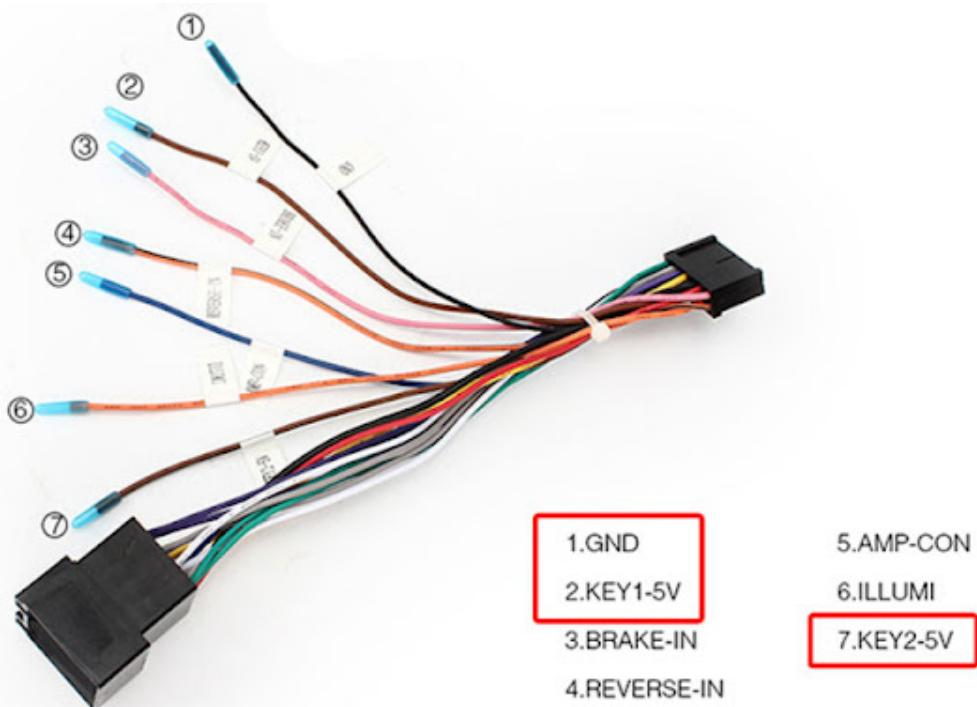
All [Pumpkin Universal 1 or 2 DIN car radio](#) are compatible with vehicles that have analogue steering controls (SWC), some additional wiring is required.
