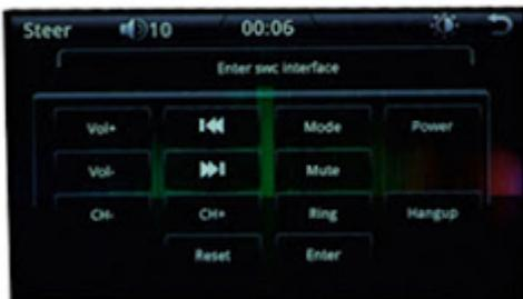
2. Push a button on the steering wheel controls, followed by the corresponding button on the head unit. Repeat this process until all required buttons are programmed.
