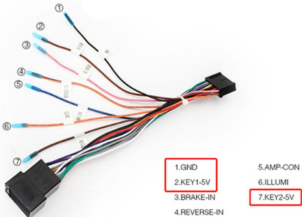
If your vehicle has digital steering controls you will require an ISO harness with steering interface and patch lead. We
