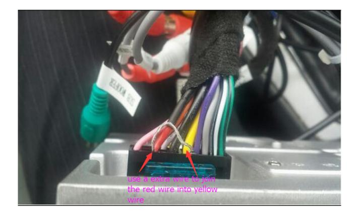
If the car stereo can be turned on with this wire modification and your car car don't have steering wheel control or you don't mind the steering wheel control, you can just connect the red wire to your ignition ACC wire, then you can continue to use the unit.
