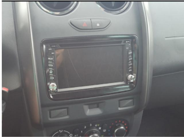
Almost all of [Pumpkin universal Andorid](#) car GPS DVD supports the Steering Wheel Control if your car came with this control from factory, but it only supports resistance ladder type since [Pumpkin](#) universal head units only offer standard ISO power cable which has no Can-Bus decoder. And the program is easy.
