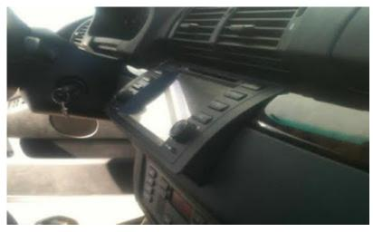
Don't worry, there are two methods which can allow you to push the new BMW X5 navigation car dvd into the dashboard fully. Some installers just cut the plastic cage, and others remove it.
