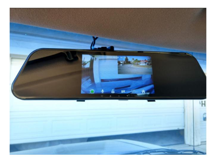
While in the Playback mode, all the various folders are accessible for front and rear recordings. These include loop recording, locked files due to impact, files due to motion close to the vehicle when parked. Only front view photos can be accessed in the Playback mode. If you take the TF card to a computer, there is also a photo from the rear camera.
