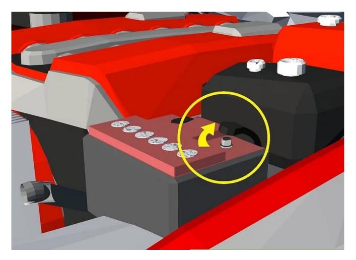
1: **Open the hood of the car and disconnect the battery.** You can disconnect the negative cable only and still be safe, but it's best to disconnect both the positive and the negative cable.
