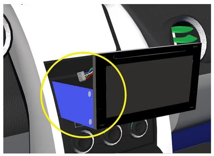
4: You can buy a wiring harness designed for your vehicle at a car audio and video equipment dealer; these are intended for aftermarket installations. Connect the wiring harness to the car's connector. See the wiring harness instructions for the proper connection.
