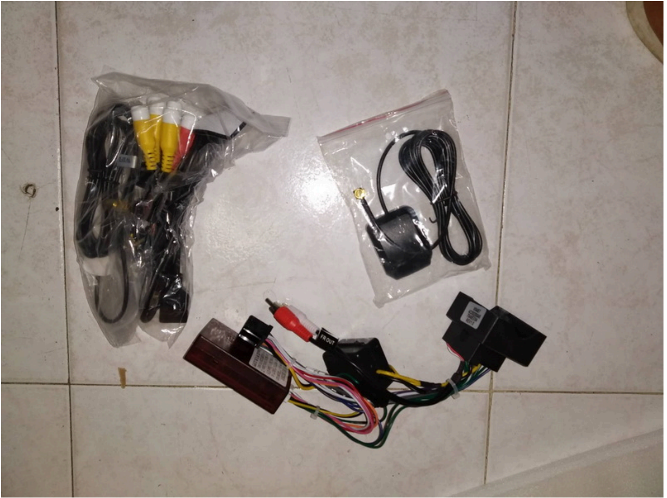
Complete wiring harnesses.
