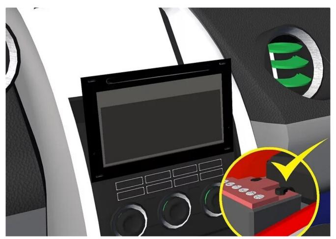
8: Replace the battery cables and make sure they are tightened. Close the hood and turn on the car. The <u>car DVD</u> player panel will light up if the installation was successful.
