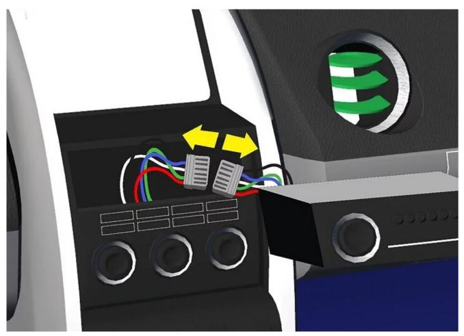
3: Carefully remove the connectors from the back of the stereo. Check the connectors to make sure they're not broken or dirty.
