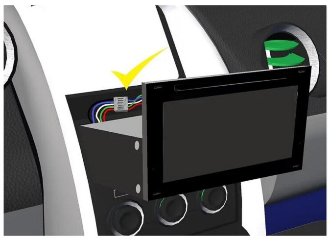
6:Connect the other end of the wiring harness to the back of the car DVD player.Connect the antenna cable to the antenna input on the back of the car DVD player.
