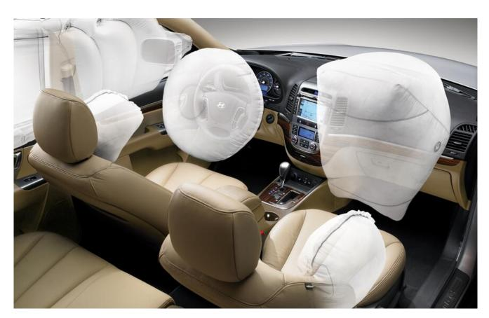
Even the least expensive cars these days have at least two front airbags. In the event of high-speed or high-impact collisions, airbags are only second to seat belts in saving the lives of front seat passengers. The latest auto
