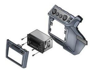
Four bolts and a pair of side brackets attach the stereo to th
