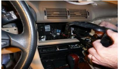
You need to pull down and slightly left the dash part which is close to the steering wheel. When you are doing this, use your other hand to push down in the middle of the opening where the cage is, and as you opened/pulled the dash/trim this far, you are able to hold it with one hand in this position and start wiggling the cage with your other hand. When are doing this, some force is necessary, but not too much. Once you start
