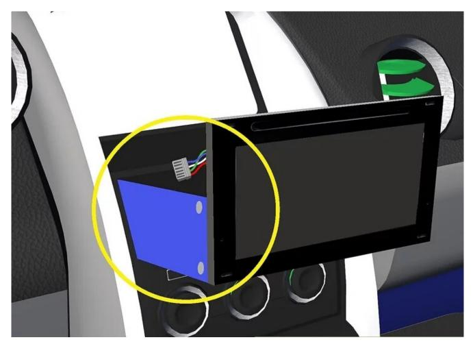
4: You can buy a wiring harness designed for your vehicle at a car audio and video equipment dealer; these are intended for aftermarket installations. Connect the wiring harness to the car's connector. See the wiring harness instructions for the proper connection.
