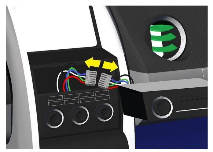
3: Carefully remove the connectors from the back of the stereo. Check the connectors to make sure they're not broken or dirty.
