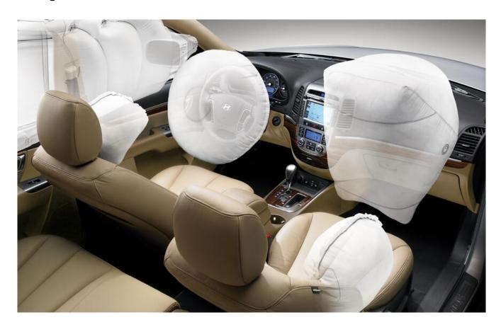
Even the least expensive cars these days have at least two front airbags. In the event of high-speed or high-impact collisions, airbags are only second to seat belts in saving the lives of front seat passengers. The latest auto technologies include airbags that deploy on the windscreen of the car to protect a pedestrian who may get hit while crossing the street.
