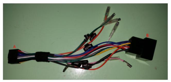
Following the photo above, the A side will be connected to <a href="Pumpkin head unit">Pumpkin head unit</a>, the B side will be connected to your car's plug which used to connect to your original car radio.
