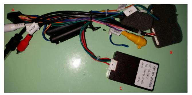
A side connects to Pumpkin autoradio dvd gps,B side connects to your car's plug,C part is the CANBUS decoder we're talking about. This CANBUS decoder controls the SWC, Turning-on/off of the head unit, parking sensor, car on-board computer and so on. Let's say it will decode and transport signal to reverse cable when the car's reversing, then the head unit can show the reversing image.
