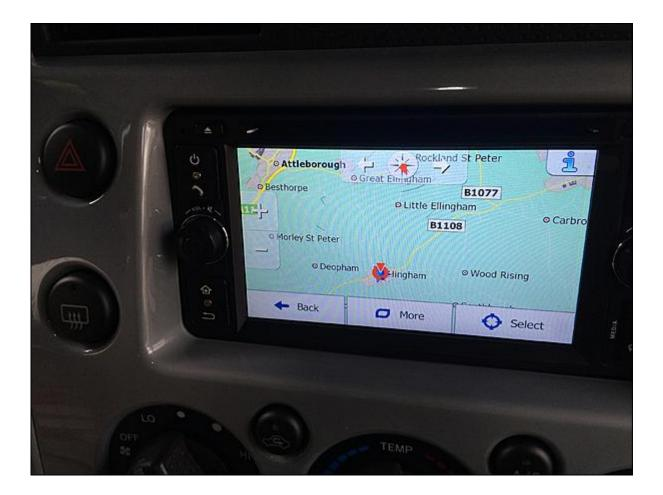
1. Check if other settings such as radio, date and time can be saved or not. If all these settings can't be saved, then you might have plugged the Red ACC cable and Yellow memory wire (labeled with B+ ) into the wrong position. Thus, there is no memory and the Android 4.4 car stereo has no data to save. All you need to do is plugging them in the right position and the setting issue will be fixed.
