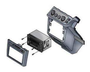
Four bolts and a pair of side brackets attach the stereo to the e dasgh in a 1998 Toyota Sienna.
