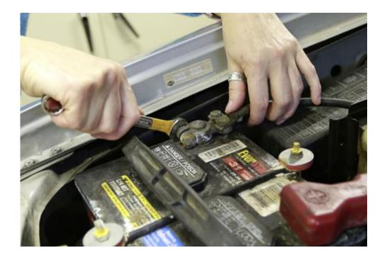
Disconnect your battery's negative terminal before any install ation job to protect your electrical system..
